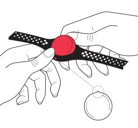
To remove, press the core out of the band. Line up the knob with the alignment hole when inserting the core into a band.
